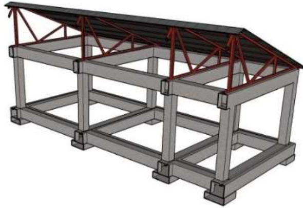
Figure 2-20: Interior view of the CGI roof (Image credit: E2E)
