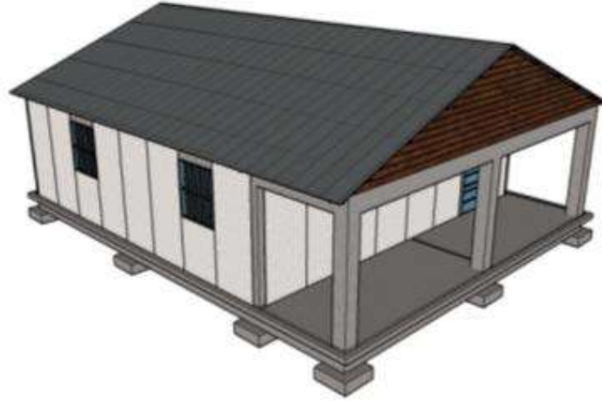
Figure 2-6: Reinforced concrete special moment frame clad with thin concrete panels (Image Source: Jensen 2016)
