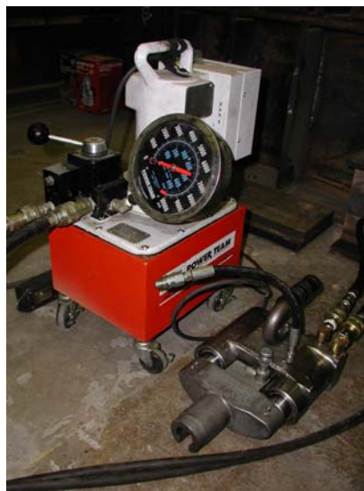
Fig. 9.16 Photograph of mono-strand post-tensioning jack and pump
