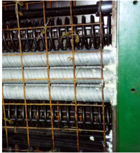
Fig. 9.11 Photograph of wall test region prior to casting of concrete
