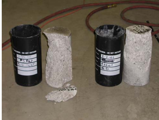
Fig. 9.27 Concrete cylinder specimens
