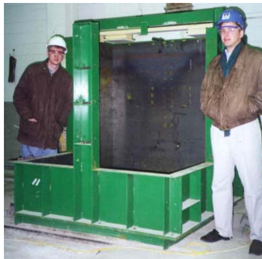
Fig. 9.7 Photograph of steel form for casting of reaction block
