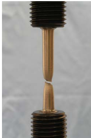
Fig. 9.18 Cover plate steel specimen
