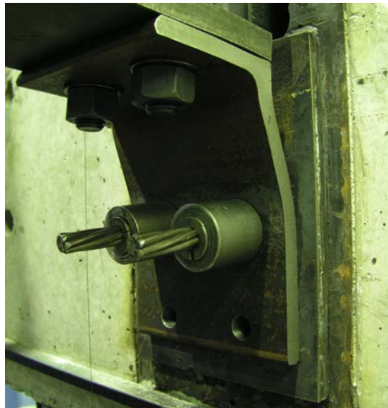
Fig. 9.14 Photograph showing angle-to-beam and angle-to-wall connections
