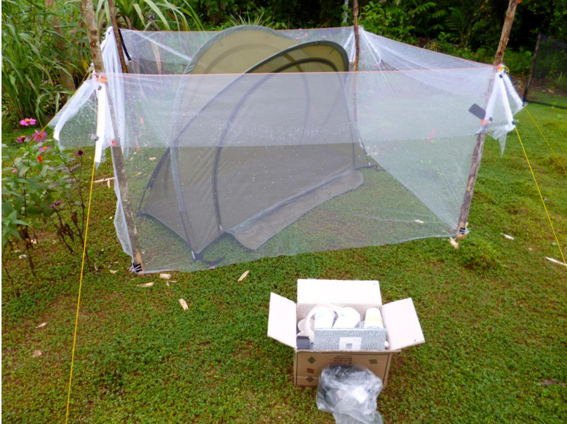
Figure 4.9 Portable mosquito tent used by the human volunteer to protect against potential bite activity during the experiment. Entry and exit are accessed through the zippered door on the lateral aspect.
