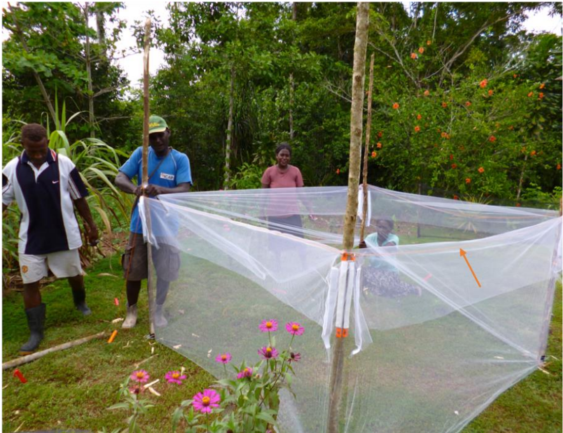
Figure 4.11 Mosquito collectors assembling a trap. Visible are the four corner poles used to frame the netting that formed the trap construct, which was held in place at a height of 0.9 m by mason line as indicated by the orange arrow. In the foreground is excess material, which when extended upwards 45° formed the eaves. These were secured in place using Velcro, and mason line for stability.
