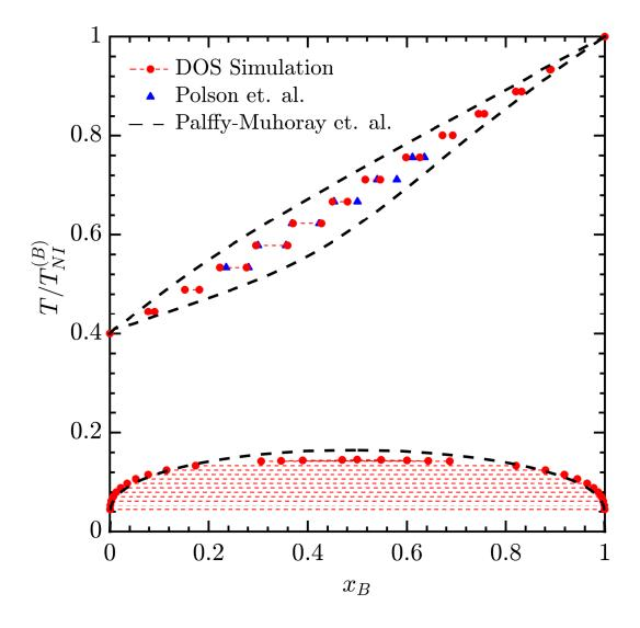
Figure 2.3. Extending the DOS approach to binary mixtures by sampling composition space  $N_A$  at a fixed  $\beta$  improves upon earlier findings [59], increasing accuracy in the NI coexistence region and permitting extension to the nematic-nematic (NN) coexistence region previously examined only in the mean-field limit [82].
