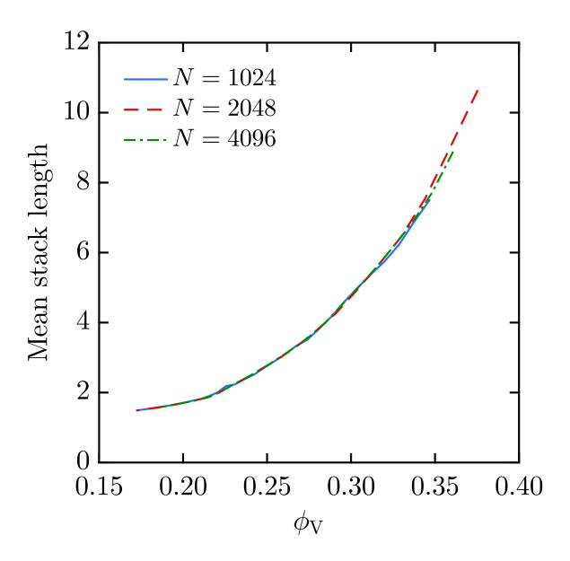
Figure 4.7. Mean stack length as a function of volume fraction  $\phi_v$  for three different system sizes at 300 K. Near–perfect agreement suggests that by N = 1024 there are little finite size effects involved in the equilibrium stack distribution.
