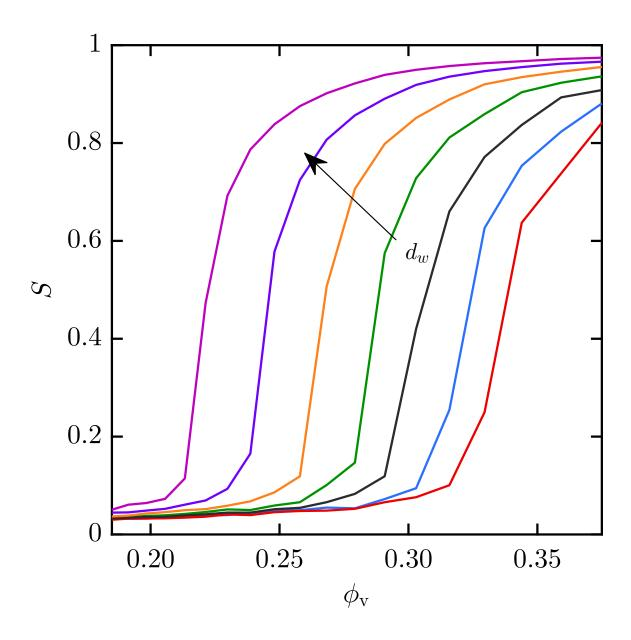
Figure 4.1. Nematic order parameter S as a function of volume fraction  $\phi_v$ at 300 K for  $d_w = 0.10, 0.15, 0.20, 0.25, 0.30, 0.35, 0.40$ . The the onset of the nematic phase occurs earlier for larger  $d_w$  due to broadening of the attractive well. The ability to easily tune  $\phi_{NI}$  allows for molecular specificity, in this case  $d_w = 0.4$  approximating the transition volume fraction of SSY.
