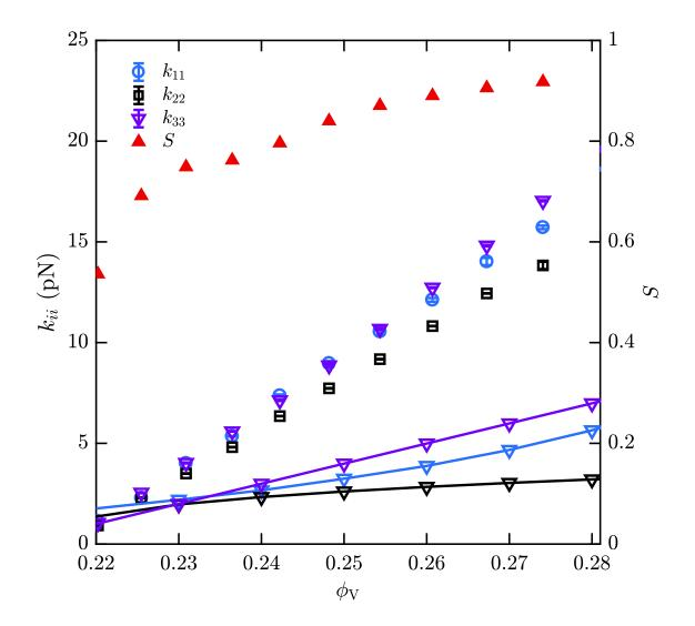
Figure 4.8. Frank elastic constants of our chromonic minimal model (open symbols) in the N phase at 300 K compared to the theory of Meyer et
