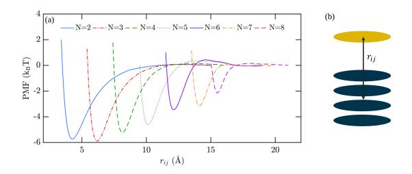
Figure 4.6. Free energy of stacking (a) obtained through PMF measurements for N = 2-8 stacks at 300 K as a function of center of mass distance between a stack and new disc (b). Dimer and trimer free energies are approximately equal and show no barrier to association. Larger stacks both exhibit an energetic and entropic penalty ( $\propto 2 \log(r_{ij})$ ) for the addition of a new disc to an existing stack.
