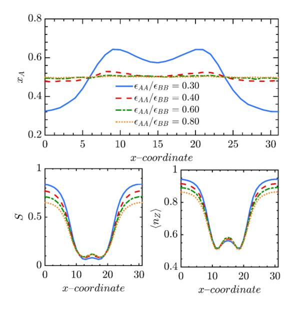
Figure 2.7. The presence of a nonlinear external field (a-c) induces segregation of a homogeneous nematic mixture. An applied Gaussian field influences the weaker elastic component to migrate to regions of high stress (a). This segregation is accompanied by decreasing nematic order (b) and
