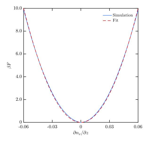
Figure 3.2. Representative parabolic free energy profile obtained using the DOS method described compared to a least squares fit. The bend elastic constant (cf. Eq. 3.14) is calculated using Eq. 3.12. This measurement was performed on the (3, 5, 2, 1) GB model at  $\rho^* = 0.338$  and  $T^* = 1.0$ .
