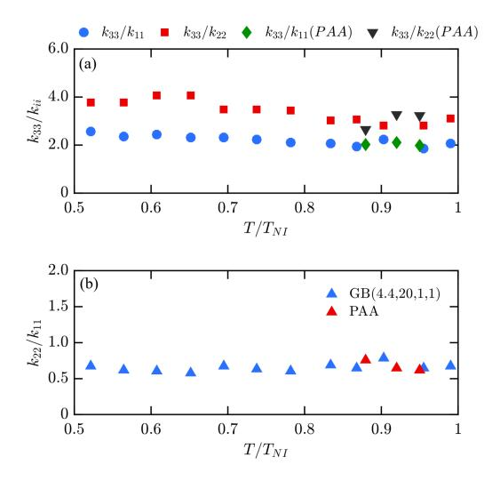
Figure 3.7. Ratio of elastic constants for the (4.4, 20, 1, 1) GB model in the nematic phase compared to PAA [153]. All three ratios, (a)  $k_{33}/k_{11}$ ,  $k_{33}/k_{22}$  and (b)  $k_{22}/k_{11}$  are approximately constant for the GB model. Excellent agreement between the GB model and PAA for all three elastic ratios.
