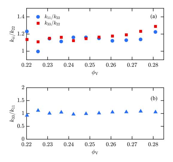
Figure 4.9. Elastic ratios for our model showing significantly less elastic anisotropy than observed experimentally.  $k_{11}/k_{33}$  is also nearly flat across concentrations which is unexpected.
