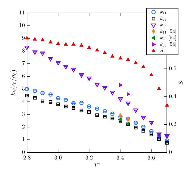
Figure 3.5. Measurements of the elastic constants for the (3, 5, 1, 3) GB model at  $\rho^* = 0.30$  compared to reported values by Humpert and Allen [124] for N = 8000. We see good agreement for  $k_{11}$  and  $k_{22}$  but measure a significantly lower value for  $k_{33}$ . The bend elastic constant is likely to be the most sensitive to finite size effects.
