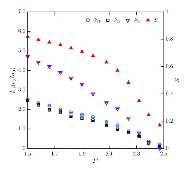
Figure 3.4. Splay, bend and twist elastic constants for the (3, 5, 1, 2) GB model at  $\rho^* = 0.301$  plotted alongside S. The elastic constants appear to vary linearly with temperature in the nematic region with a more significant drop at the NI transition, an effect which is most prominent in  $k_{33}$ .
