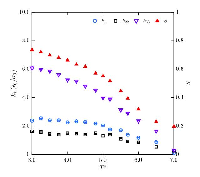
Figure 3.6. Elastic constants and order parameter S for the (4.4, 20, 1, 1) GB model at  $\rho^* = 0.193$ . Unlike the (3, 5, 2, 1) and (3, 5, 1, 2) models, this shows significant  $k_{11}$ ,  $k_{22}$  separation. Both  $k_{11}$  and  $k_{22}$  also remain nearly constant until the onset of the NI transition with  $k_{33}$  roughly tracking S.
