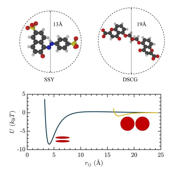
Figure 4.2. Approximate diameters of SSY and DSCG chromonic liquid crystals used to develop the Gay–Berne coarse grained model. The potential shown represents the effective interaction between two 16.27 Å diameter discs in face–face and side–side orientations.
