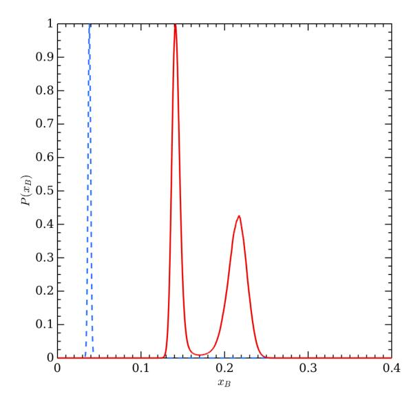
Figure 2.2. Probability distribution of a LL binary mixture with  $\epsilon_{AA}/\epsilon_{BB} = 0.35$  at  $T^* = 0.50$ . The dashed blue line represents  $P(x_B)$  at a starting guess of  $\mu = 2.0$ . Coexistence was identified by numerically determining the position of two peaks in probability, and automatically adjusting the chemical potential until the integrated areas under these peaks were equal. The solid red line represents that final value,  $\mu_{eq} = 1.451$ .
