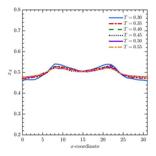
Figure 2.8. The compositional segregation resulting from external nonlinear stress responds weakly to changes in temperature. For  $\epsilon_{AA}/\epsilon_{BB} = 0.40$  there is little change in profile of  $x_A$  throughout nearly the entire homogeneous nematic regime.
