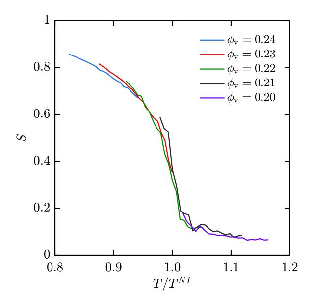
Figure 4.10. Nematic order parameter as a function of scaled temperature for various volume fractions at 300K illustrates universality in  $P_2$ . This is consistent with observations in Ref. 185. Due to finite size effects,  $P_2$  does not equal zero in the isotropic regime.
