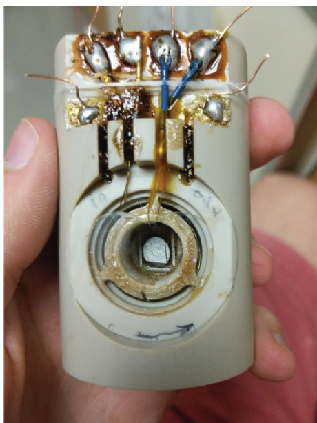
Figure A.3. Mk 2 resistive field coil. Coil has a much larger external diameter than the Mk 1, making it only suitable for cryomagnets with bore \phi \geq 50 mm. Mounted inside the coil is the large, roughly cylindrical crystal of MnSi used ILL and ORNL.
